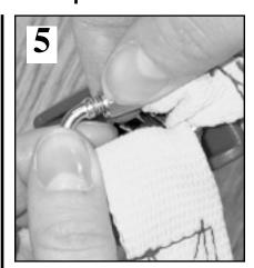
5. Lock oval locking link by screwing clip closed. Finger tighten.
