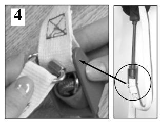
**4.** Thread oval locking link through the loop of the adjustment strap located at the bottom end of the bungee cord.
