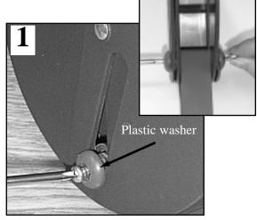
1. Using a phillips screwdriver, remove metal screw and plastic washer from door frame clamp where bungee cord is attached. Use a coin (penny or dime) to hold plastic screw on other side of door frame clamp in place.
